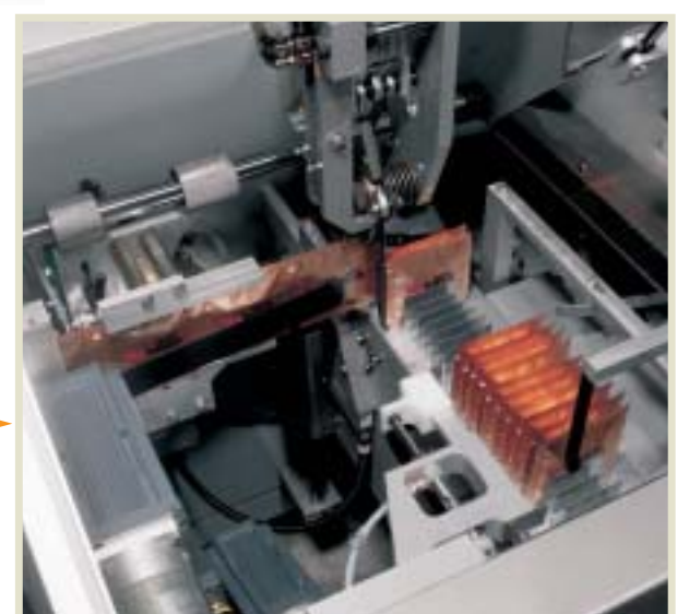
Outer envelope cutting and stacking
