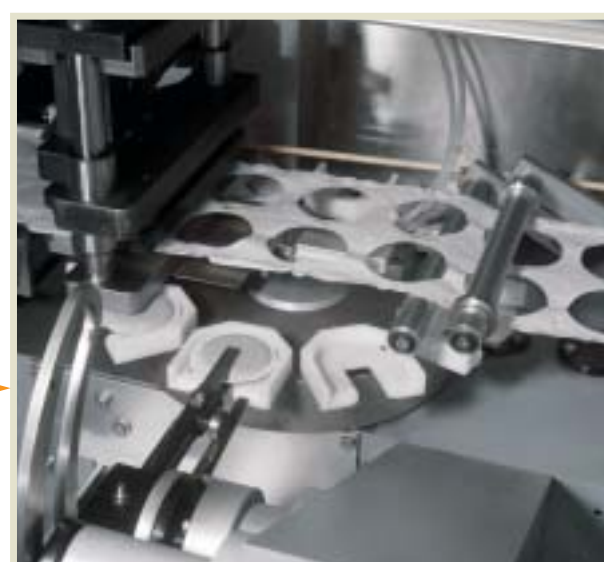
Pod removal from transfer wheel
